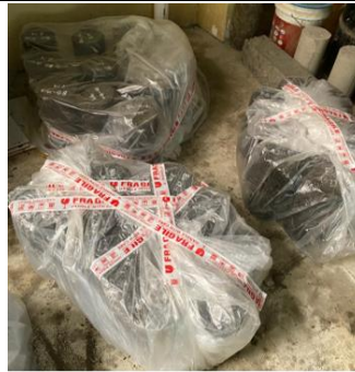
Gambar 2. Metode Perawatan Beton Geopolimer
