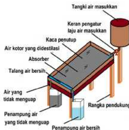
Gambar 1. Model distilasi air jenis absorber kain
