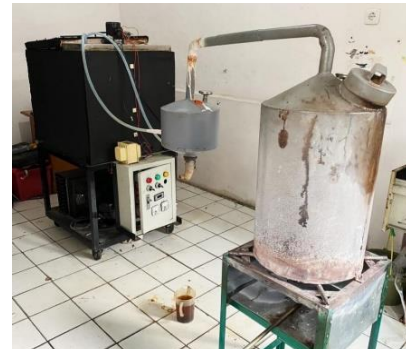
Gambar 3: Reaktor, tabung distilasi, mesin brine cooling
