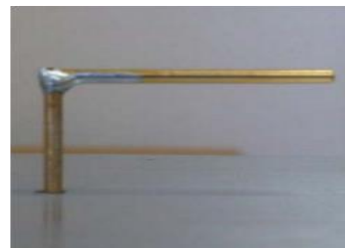
Gambar 2.3 Struktur Dasar L-probe (H-Shaped Microstrip Patch Antenna Using L-Probe Fed For Wideband Applications: IEEE, 2012)
