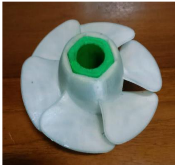
Gambar 5. Hasil 3D Sudu Turbin propeller
