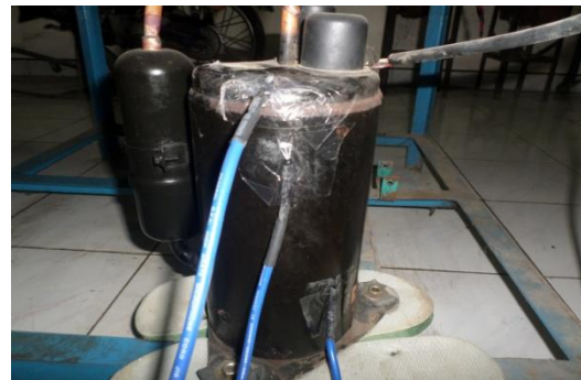
Fig 10. Experiment Measurement of the temperature in the Compressor Motor
