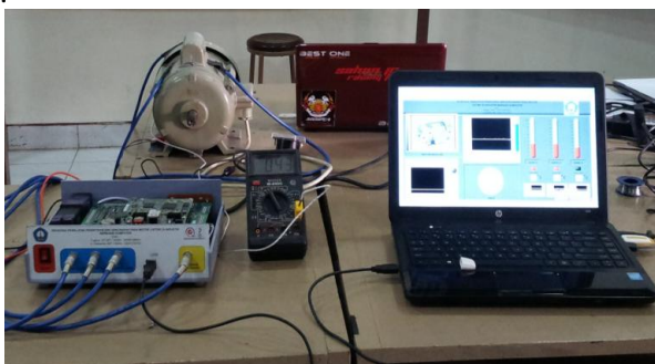
Fig 4. Hardware on early detection of damage the electric motor based computer
