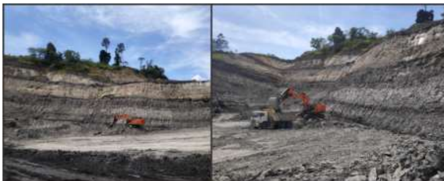
Gambar 3. Proses coal cleaning ( overburden removal ).
