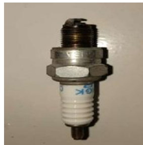
Gambar 3. Busi Standar NGK (CR6HSA)(0,6mm,0,7mm,0,8mm)
