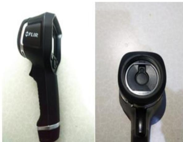
**Gambar 3** Kamera *thermal imaging*
