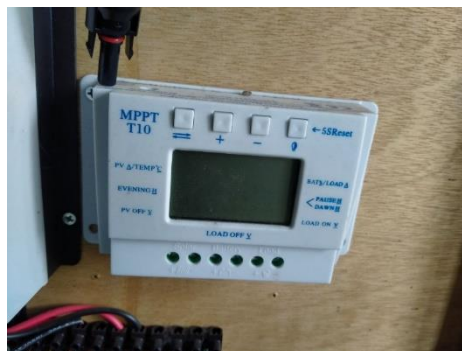
Gambar 6. Gambar Solar Charge Control Pulse Width Modulation (SCC PWM)
