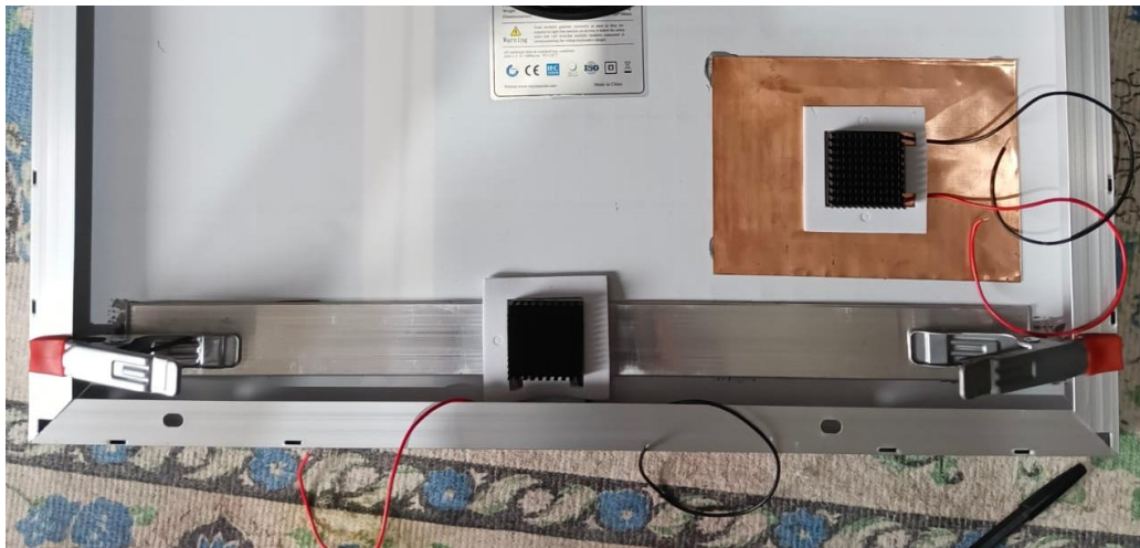
Figure 3 TEG System with MCHP (Bottom) and Copper Plate (Top)
